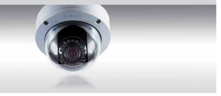
The WZ45 Integrated Day/Night Dome camera is a vandal-resistant, user-friendly surface mount camera designed for effective 24/7 surveillance. Equipped with a 540 TVL mechanical filter CCD and 18 high-efficiency infrared LEDs, the camera delivers vivid daytime color and 18 m (60 ft) of active-infrared night vision.
